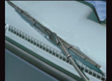
**Wipers with integrated washer nozzles**
